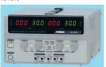
Laboratory grade power supply provides adjustable 0-30V DC output, and 0-3A adjustable current limiting, on each of two isolated channels. Four independant three-digit LED displays simultaneously show output voltage and current for each channel.
